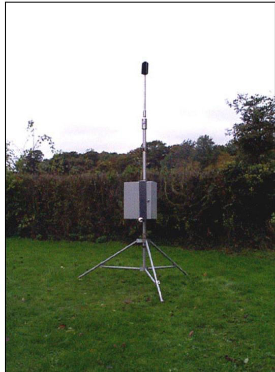
**Figure 5** 3.5 m NTK Mobile Monitor
