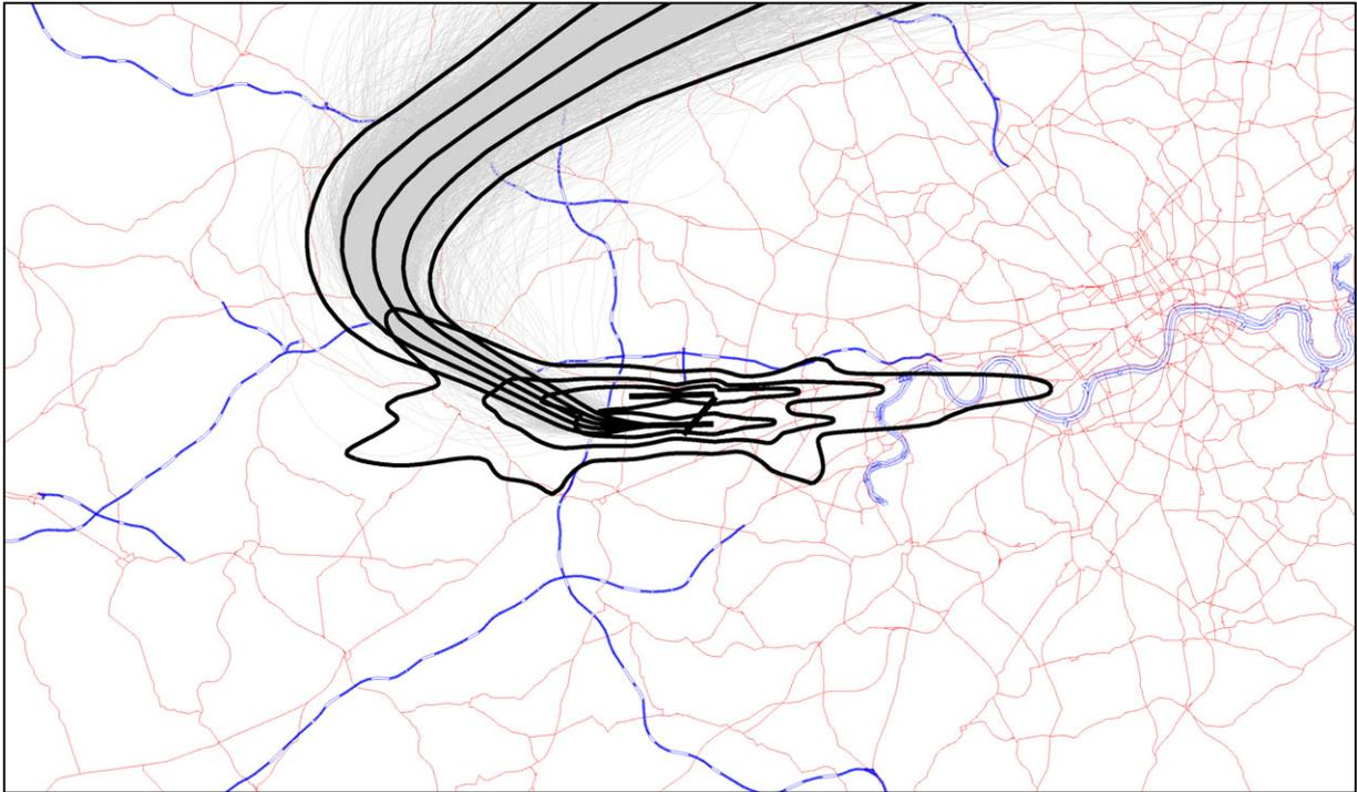
**Figure 10** Example of Mean and Dispersed Departure Tracks
