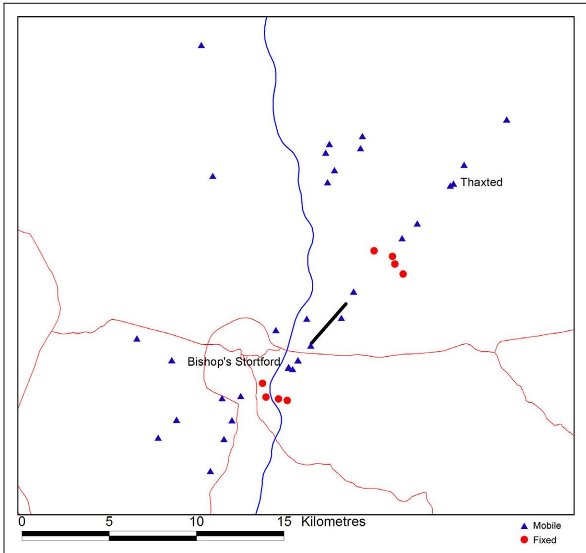
**Figure 3** Location of Fixed and Mobile Noise Monitors Around Stansted
