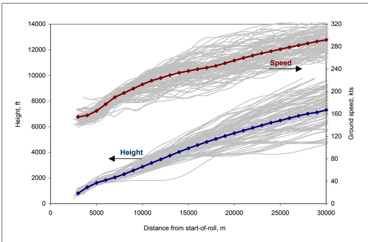
**Figure 9** Example of Mean Departure Height and Speed Profiles (for Boeing 757-200 aircraft, with underlying radar data shown)
