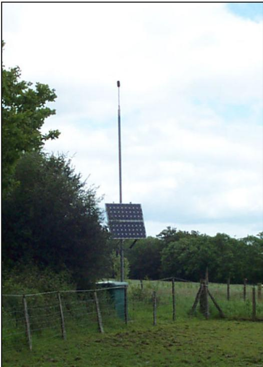
**Figure 4** 6 m NTK Fixed Monitor (fitted with solar panels)
