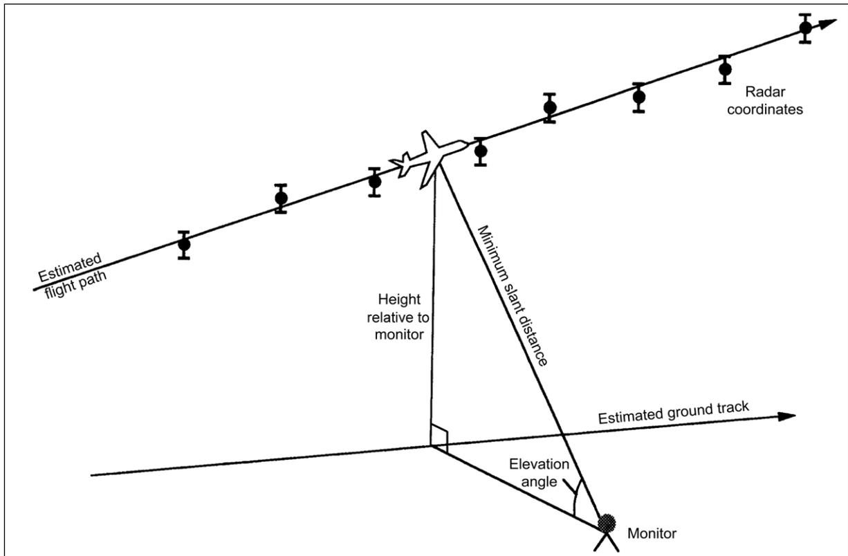
**Figure 8** Calculation of Source-to-Receiver Geometry
